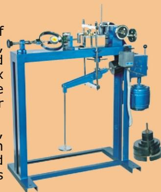
♦ **Shear Box Assembly for Square Specimen:** Comprising Direct Shear box in two halves for a square specimen size 60 x 60 x 25 mm one pair of plain gripper plates, one pair of perforated gripper plates, one pair of porous stones, one top loading pad. Shear box housing: Accommodates the Direct Shear Box assembly.
